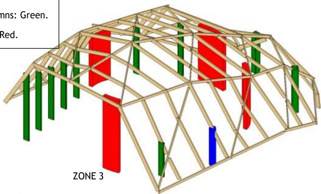
**Bracing for diaphragm action**
