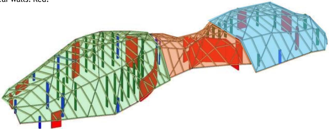
The entire pavilion is split longitudinally into 3 zones as marked above. Each zone has its own structural system for gravity and lateral loads.
