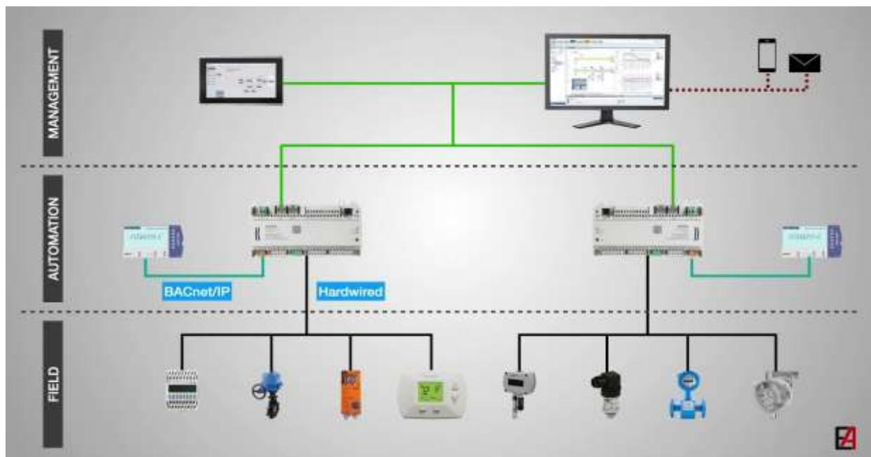
Picture: Schematic of Building Management System (BMS)
