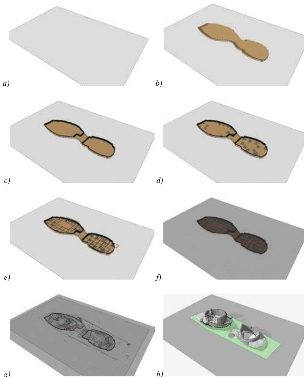
**Figure 1: Floating Foundation Workflow. a) Ground Level, b) Excavation of Soil Weight  $\geq$  Building Weight, c) Peripheral Retaining Wall & Thin raft with inverted beam at base, d) Column erected from inverted beam based on column layout, e) Tie Beam at Ground Level, f) Flooring, g) Ground Level, h) Super Structure**
