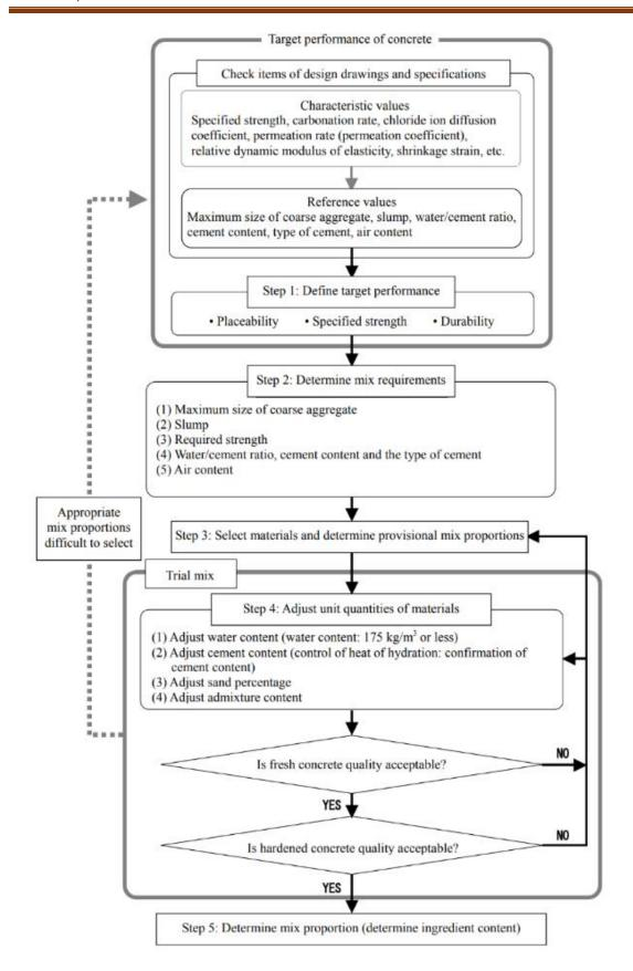
Figure 1: Concrete Mix Design workflow (Ref. JGC16\_Standard\_Specifications\_Materials\_and\_Construction)
